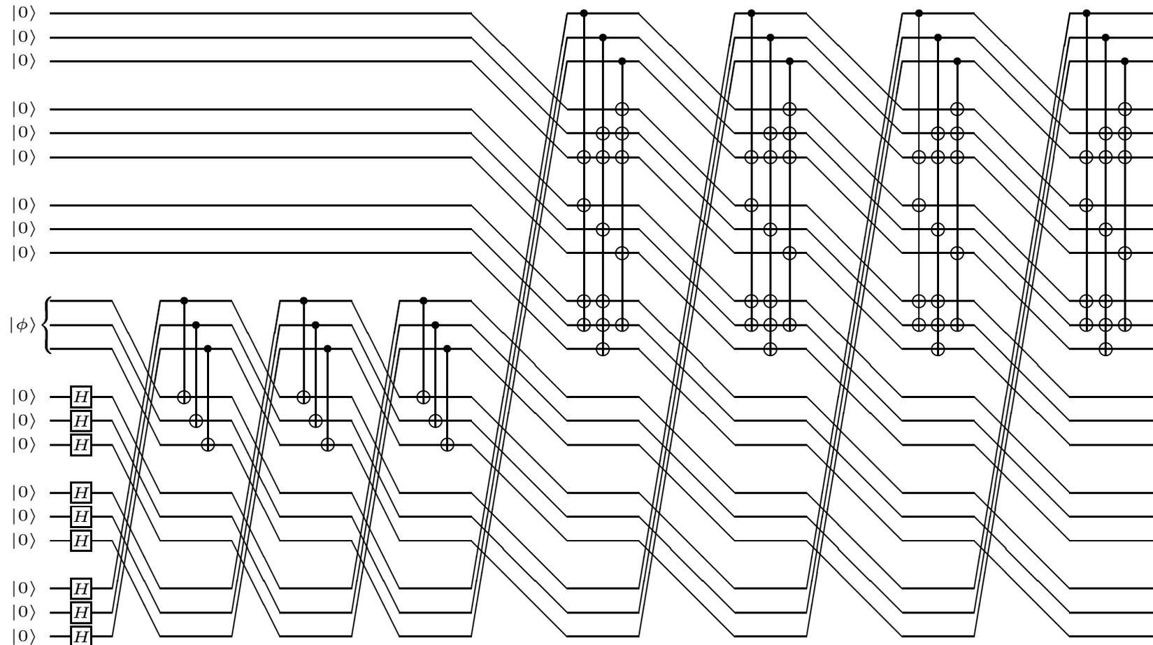
Encoder for the quantum Reed-Solomon code  $[[21, 3, 5]]$  using quantum shift registers for the multiplication by  $\tilde{g}(X) = X + 1$  and  $g^\perp = \alpha X^3 + X^2 + \alpha^2 X + 1$ .
